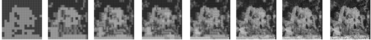
Figure 8: The reconstructed left image “Aqua” size 64x64 pixels in 1- 8 bits respectively based on QVQ technique using haar wavelet
