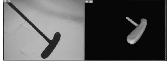
Figure 2: Left is the original image of a golf head. Right is the reconstructed result in 3D.
