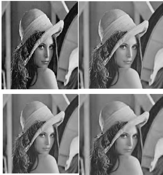
Figure 3: Simulation results using wavelet transform.(a) Original test image (top left). (b) Compression ratio 16:1, PSNR=32.50 (top right). (c) Compression ratio 35:1, PSNR=27.34 (bottom left). (d) Compression ratio 64:1, PSNR=24.77 (bottom right).
