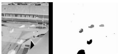
Figure 2: Object detection in a traffic scene (left: original image, right processed image).
