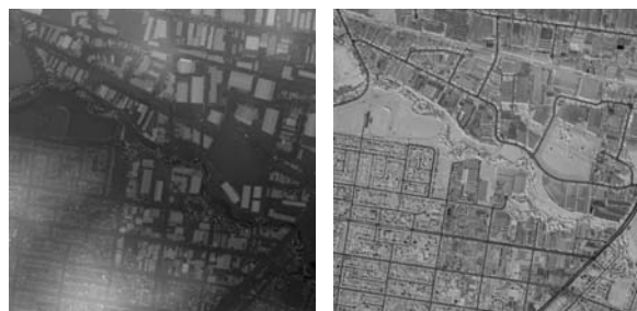
Figure 2: The test site. Left: DSM (black: low areas, white: high areas). Total area: 2000 \times 2000 \text{ m}^2 . Right: The “pseudo-NDVI-image”.
