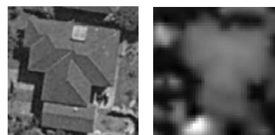
Figure 4: One of the buildings in the test dataset. Left: Digital orthophoto (resolution: 15 cm). Right: DSM.
