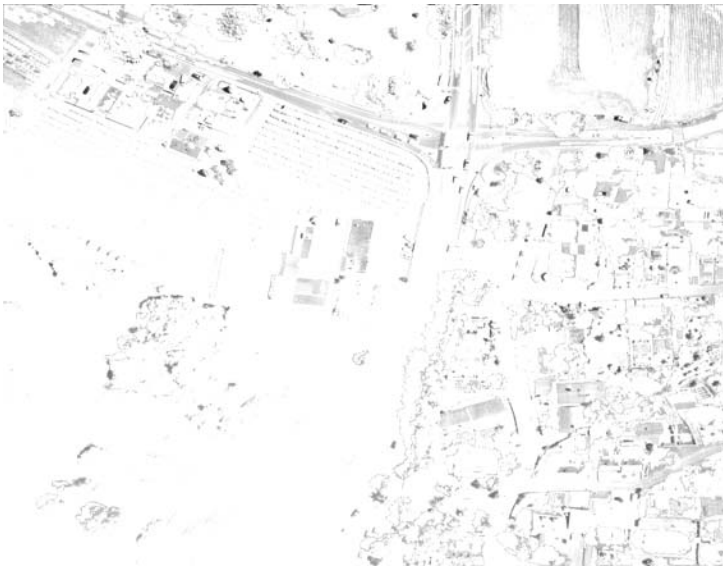
Figure 5: Separation of roofs, trees, bushes and lawn by texture analysis of image of fig. 4
