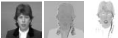
Figure 1: From left to right: an image extracted from the Claire sequence, the corresponding angular hue and the logarithmic hue-like image obtained using the LUX space.
