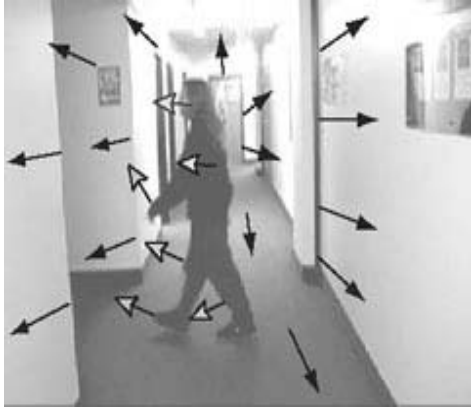
Fig. 2 Motion in a scene. The dark arrows show background motion generated from the motion of the camera. The white filled arrows show the motion of the human.
