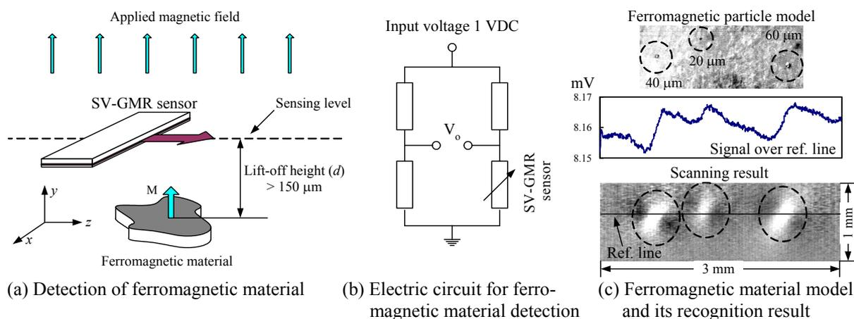
(a) Detection of ferromagnetic material (b) Electric circuit for ferromagnetic material detection (c) Ferromagnetic material model and its recognition result
