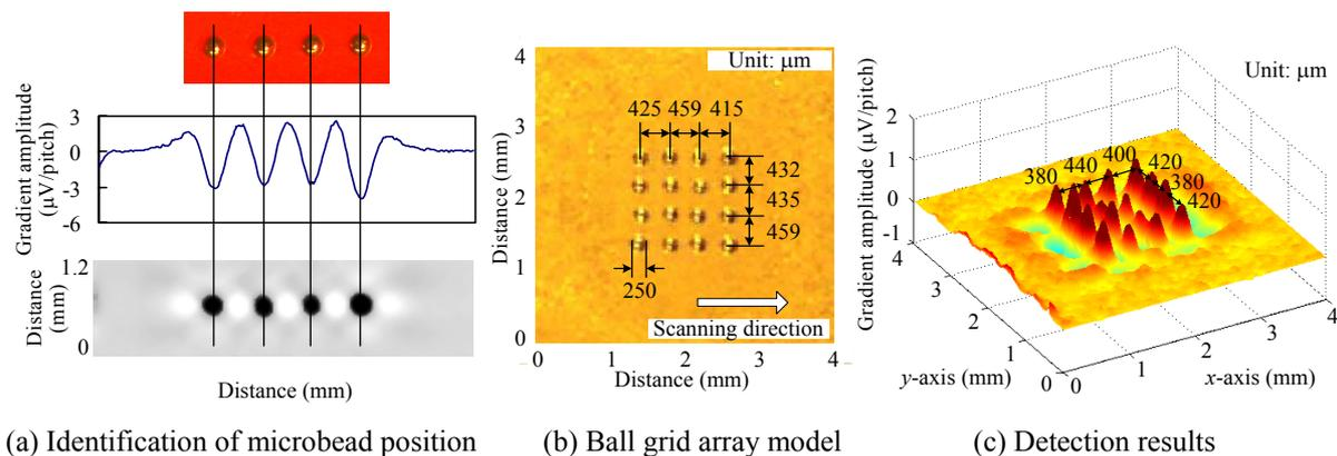
(a) Identification of microbead position (b) Ball grid array model (c) Detection results
