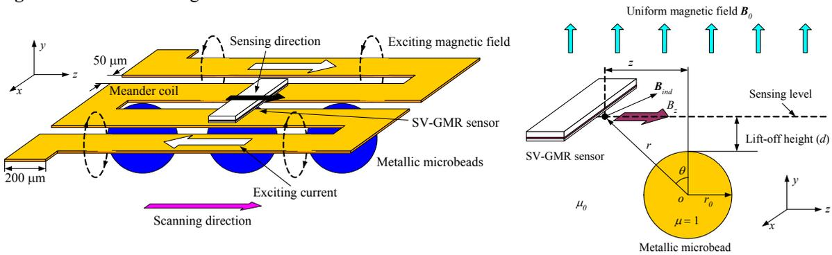
**Figure 2:** Proposed ECT probe structure with SV-GMR sensor (left) and magnetic field analysis model (right).
