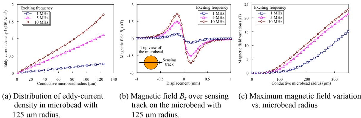
**Figure 3:** Analytical results of magnetic field occurred from eddy-current flowing in the microbead placed under uniform magnetic field  $B_0 = 100 \mu\text{T}$  and lift-off height of 162  $\mu\text{m}$ .
