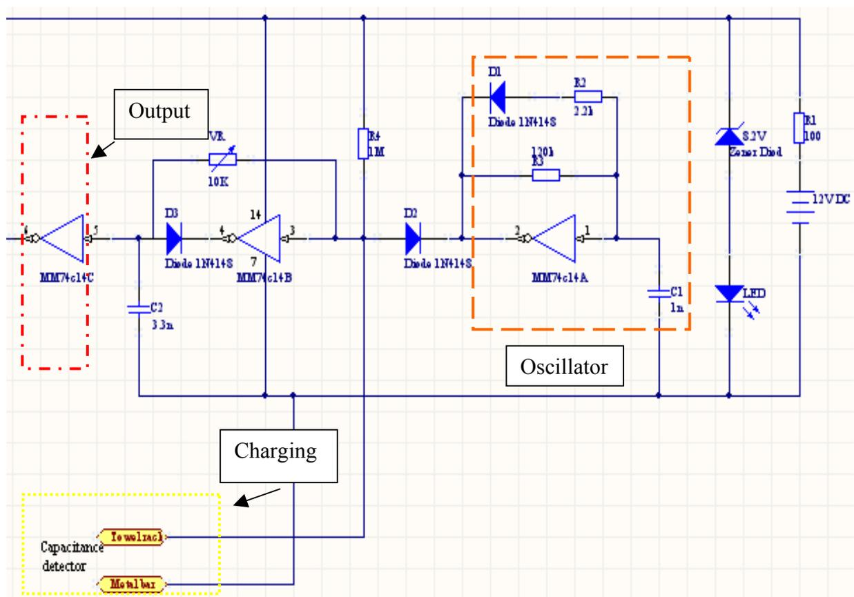
Figure 4. Capacitance to voltage converter
