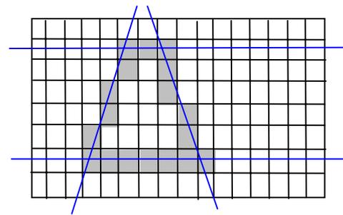
Figure 4: Grouped Edge detected pixels and candidate lines in object
