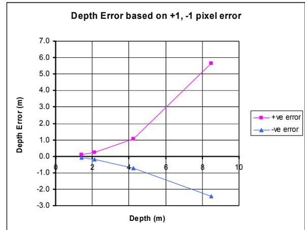
**Figure 6:** Variation in Depth measured due to  $\pm 1$  pixel error in object's position
