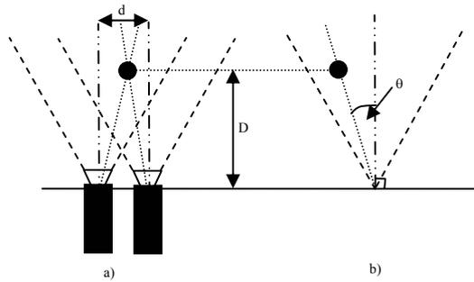
**Figure 5:** a) Stereo Cameras with object in field of view at depth  $D$  and interocular distance  $d$ . b) Angle of object ( $\theta$ ) relative to perpendicular to epipolar line.
