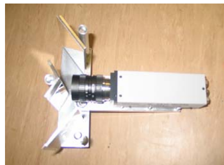
Figure 12: The completed catadioptric system.
