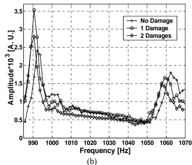
**Figure 4.** Comparison between the FRF's (a) and SFRF's (b) amplitudes for the 992 and 1060Hz resonant frequencies.
