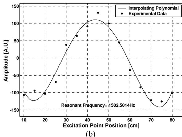
**Figure 2.** Comparison between vibrational shapes belonging to the mode at 1502Hz, (a) vibrometer, (b) FBG.
