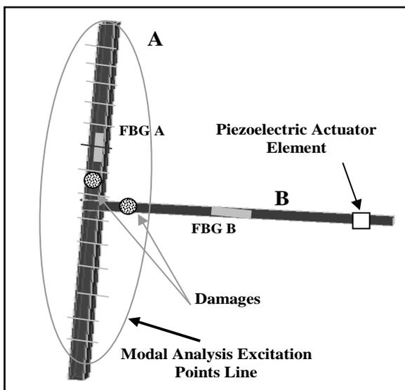
Figure 1: A scheme of the test structure.
