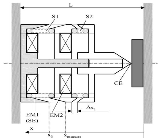
Fig.1: Sketch of the proposed distance sensor with self-calibration capability
