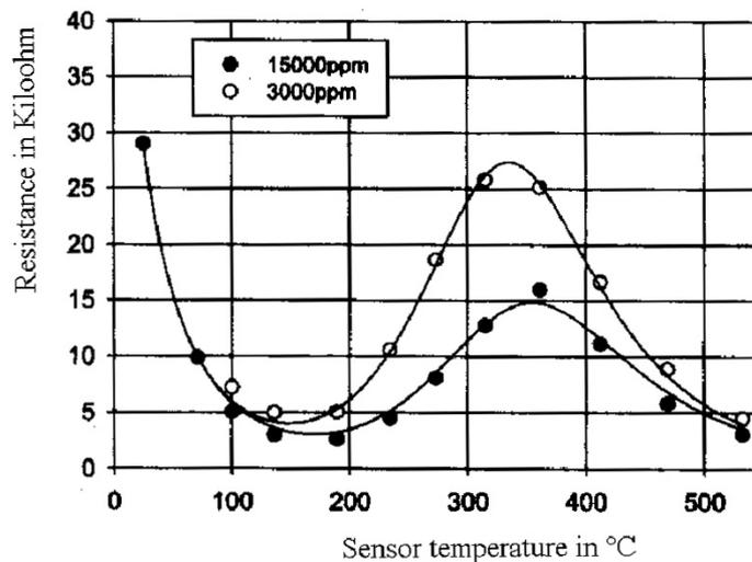
Fig. 2: Typical resistance of a semiconductor gas sensor as a function of temperature with humidity as the parameter: Measured points and modeled function of of the sensor resistance in dependence of the temperature and humidity for the gas concentration  $x = 0$  ppm [15]
