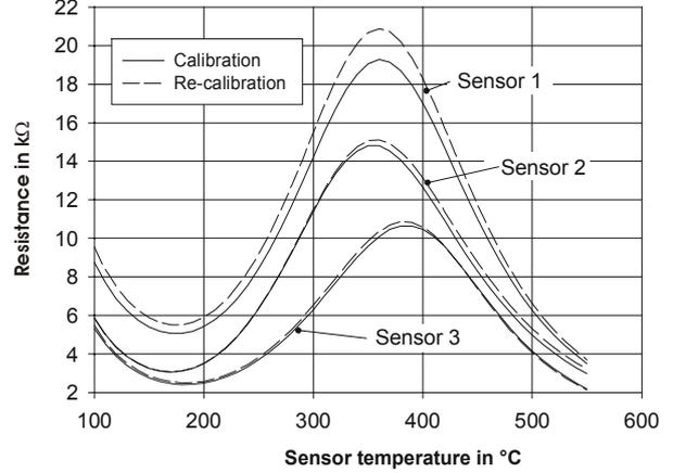
**Fig. 3.** Results from the re-calibration of the zero-point of semiconductor gas sensors at humidity level assumed as unknown (15000 ppm in this case).
