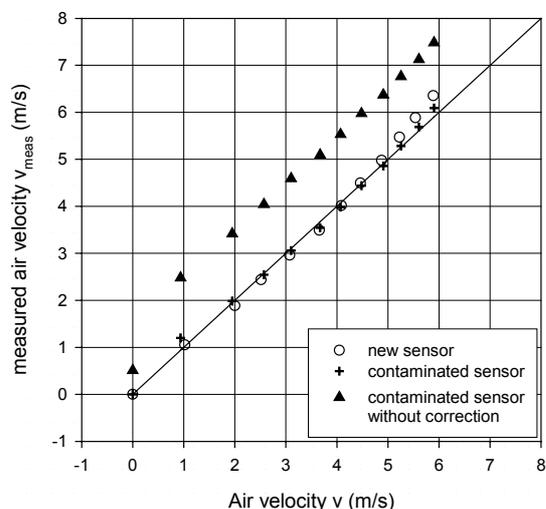
Fig. 4. Measured air velocity against real air velocity with and without the described model-based correction
