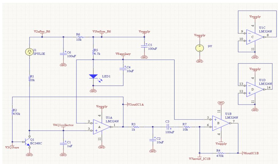
**Figure 3:** Simulated circuit of proposed system
