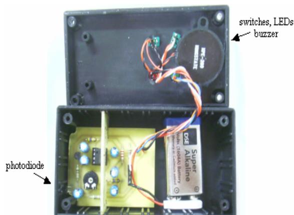
Figure 10: Interior of the designed detector black box encompassing PCB
