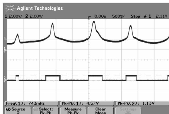
**Figure 8:** Pulses caused by direct movement of the hand in front of the photodiode
