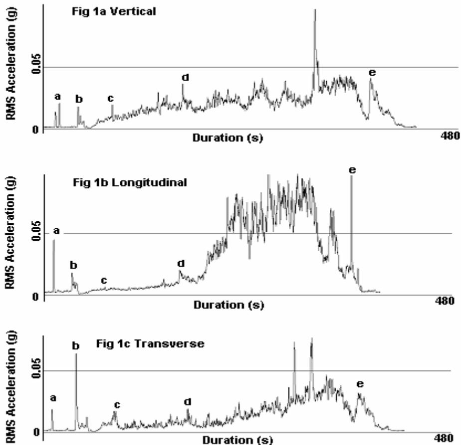
For the aircraft tests a plot of RMS vibration versus time is plotted for each axis. These are shown in Figure 1
