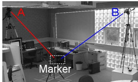
**Figure 6:** Experimental setup (two cameras and the marker).
