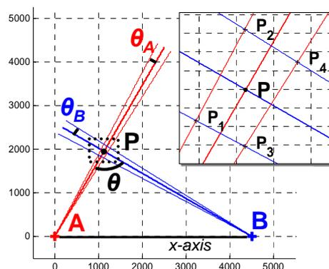
**Figure 2:** Triangulation error: the region delimited by the points  $P_1, P_2, P_3,$  and  $P_4$  illustrates the shape of the uncertainty region. The position error of the reconstructed points comes from the intersection of error cones. The maximum error lies in the plane ( $ABP$ ).
