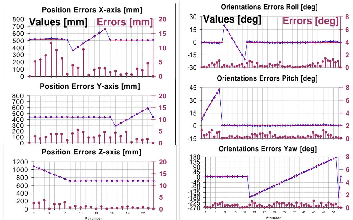
**Figure 7:** Results of the 3DOF position and 3DOF orientation computation with the stereoscopy-based pose estimation method.
