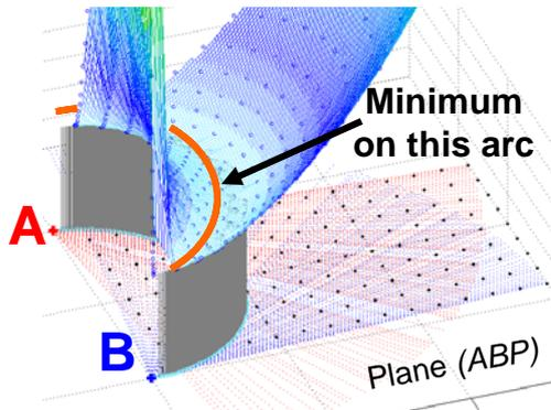
**Figure 3:** Estimation of the triangulation error. Points  $P$  are sampled on a  $5 \times 5\text{mm}$  grid in the plane  $(ABP)$ ; the angle  $\theta$  varies within the range  $]0,\pi[$ . A minimum triangulation error of  $\pm 8\text{mm}$  is reached for  $\theta_0=\pi/2$ , independently of variations in  $\overline{AB}$ ,  $\theta_A$ , and  $\theta_B$ .
