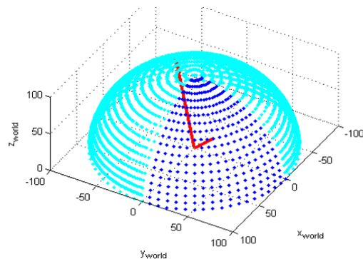
**Figure 4:** Estimation of the optimal stereo vision system orientation. The dots indicate the location of the sampled orientations. Simulations were performed for  $\phi_A$  and  $\psi_A \in [0, \pi/2]$ . The solid lines represent the optical axes of the cameras in their optimal positions.
