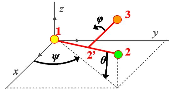
**Figure 5:** The orientation  $r=(\varphi,\theta,\psi)$  of the rigid marker.  $r$  is defined by the 3D position of the three spherical targets in the world reference frame.  $\varphi$  and  $\theta \in [-\pi/2,\pi/2]$ , and  $\psi \in [0,2\pi]$ .
