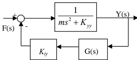
Figure 1: Block diagram of AMB system in one axis
