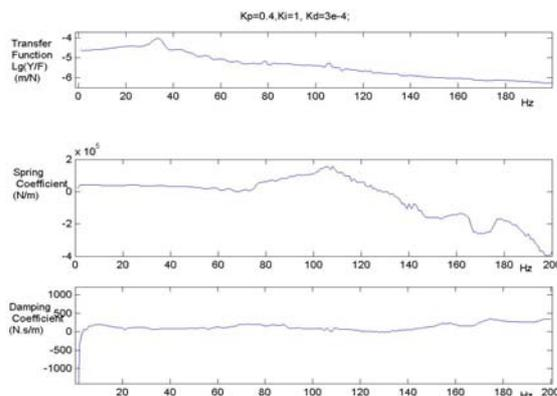
Figure 5: Actual stiffness and damping coefficients of electromagnets
