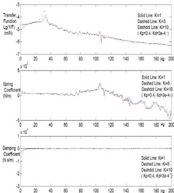
Figure 6: Characteristics of electromagnetic actuator with varying integral feedback
