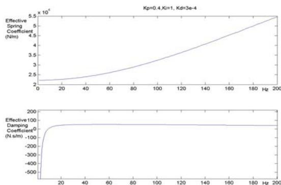
Figure 4: Effective stiffness and damping coefficients of electromagnets
