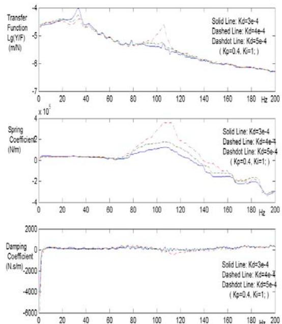
Figure 8: Characteristics of electromagnetic actuator with varying derivative feedback
