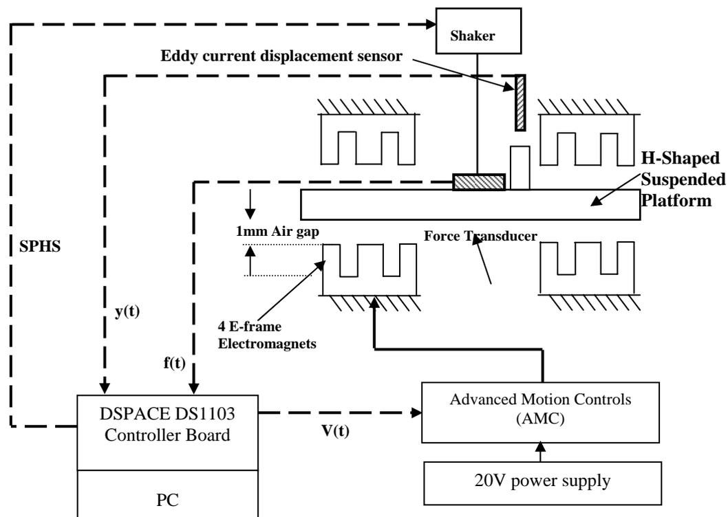
Figure 2: Instrumentation arrangement of experiment
