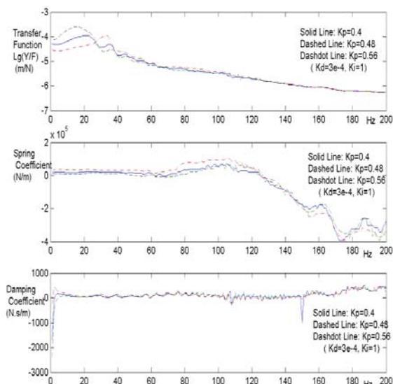
**Figure 10:** Characteristics of electromagnetic actuator with varying proportional feedback
