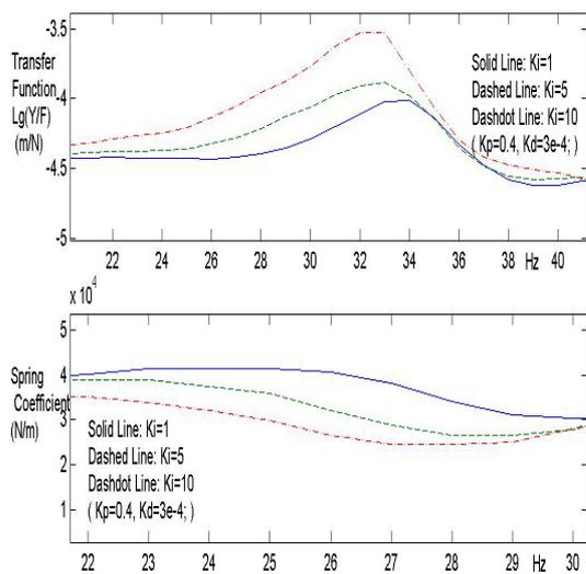
Figure 7: Expansion of Figure 6 around natural frequency
