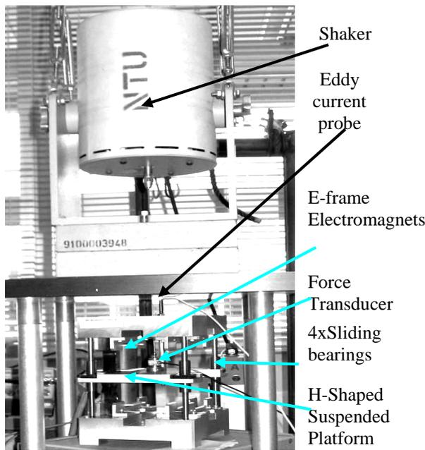
Figure 3: Photo of experimental setup
