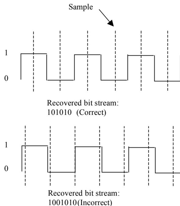
**Figure 2:** (a) Received data waveform being sampled at the correct time. (b) Received waveform being sampled at incorrect frequency and phase.
