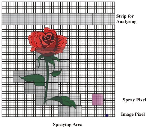
**Figure 4:** Concept diagram for image pixel, spray pixel and spray pattern
