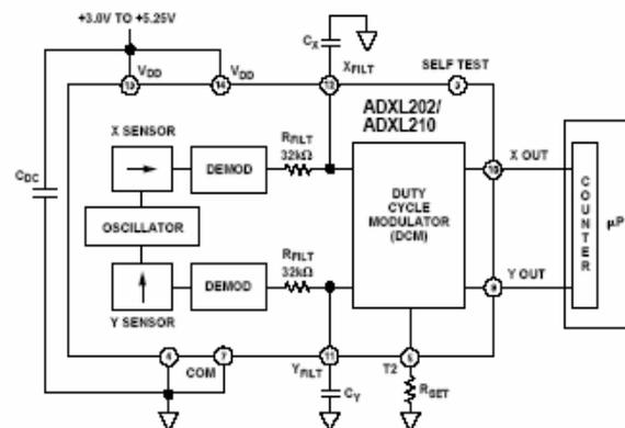
Figure 1: Function block diagram of ADXL202 [14]
