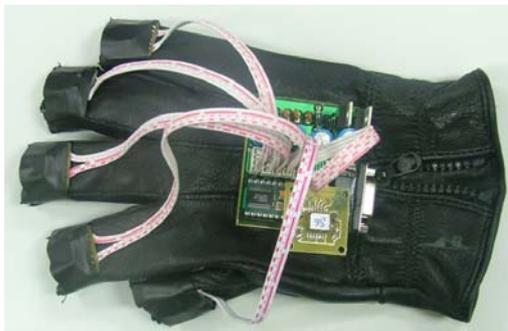
**Figure 2:** Sensing Glove with six accelerometers and Basic Stamp microcontroller.
