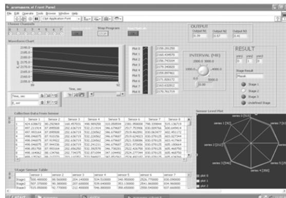
Figure 2: Graphical User Interface (GUI) for electronic nose system
