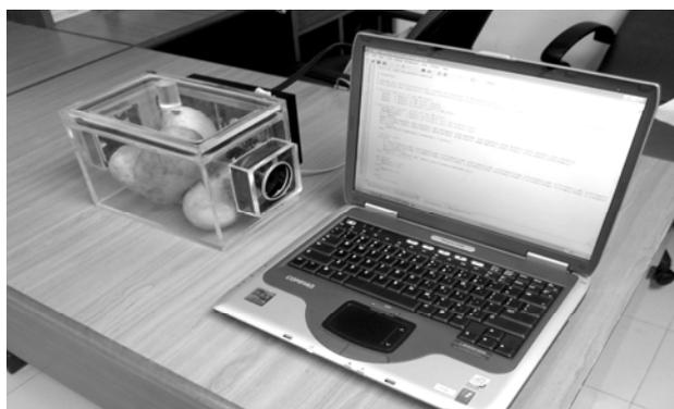
Figure 1: the experimental set-up used to analyze the aroma of *Harumanis*
