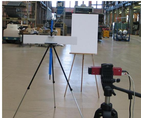
Figure 4: Experimental setup to determine the effect of mixed pixels on flash lidar devices
