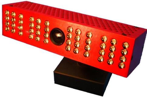
Figure 1: The CSEM SwissRanger2 flash lidar device
