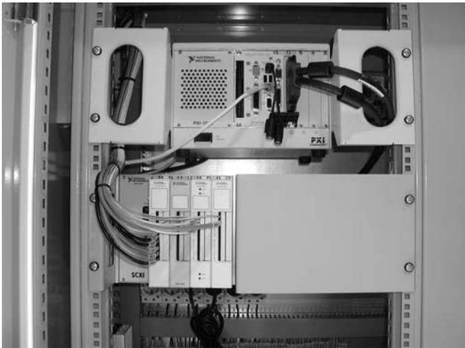
Fig. 3. Operating implementation of the PXI (topmost) and SCXI (just below) chassis.
