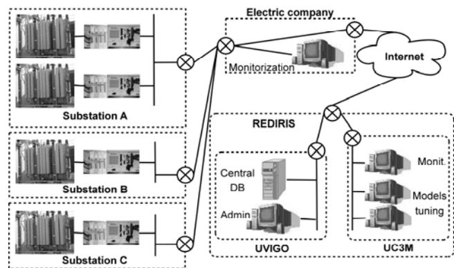
Fig. 5. Network infrastructure of the four clone systems installed
