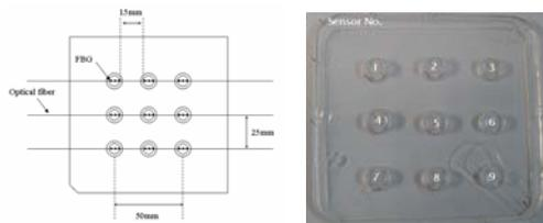
Figure 14 3x3 array sensor
