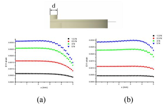
**Figure 6** Strain distribution of different diameters of the contact mesa when (a)  $d = 4\text{mm}$ , and (b)  $d = 5\text{mm}$
