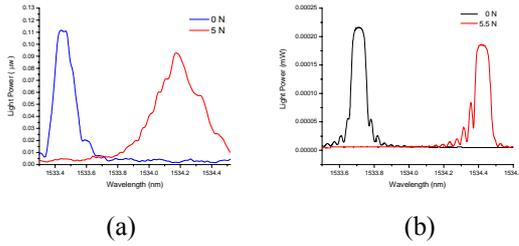
**Figure 8** Experimental verification that chirping is minimized: (a) chirping, (b) minimized chirping
