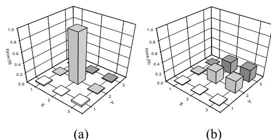
**Figure 16** Evaluation of 3x3 array sensors: (a) 1N on 5<sup>th</sup> taxel of diaphragm type sensor array, (b) 1N on 5<sup>th</sup>, 6<sup>th</sup>, 8<sup>th</sup>, 9<sup>th</sup> taxels of diaphragm type sensor array
