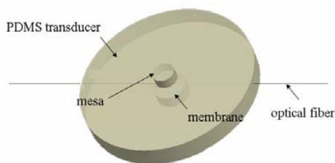
**Figure 4** Structure of the flexible force sensor
