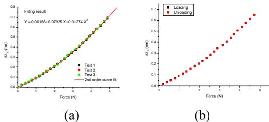
Figure 13 Experimental verification of the prototype sensor: (a) repeatability of diaphragm type sensor, (b) hysteresis of diaphragm type sensor
