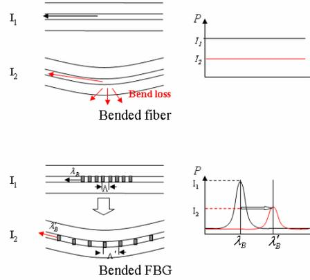
**Figure 2** Micro bending effect of Bragg wavelength
