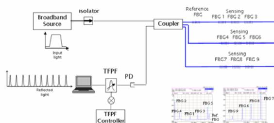
Figure 15 Interrogation system of the 3x3 array sensor
