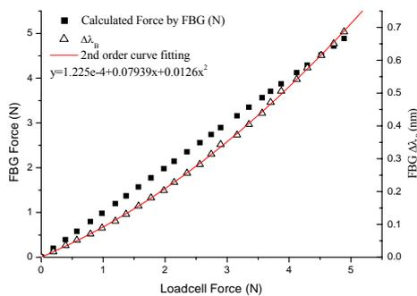
Figure 12 Plots of Bragg wavelength shift and prototype force signal vs. load cell signal
