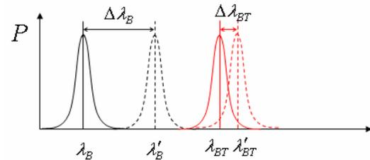
**Figure 11** Temperature compensation of flexible force sensor
