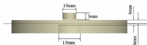
**Figure 7** Dimensions of the prototype flexible sensor
