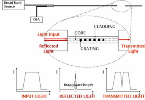
**Figure 1** Fiber Bragg Grating sensor encoding operation
