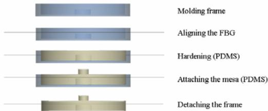
**Figure 9** Fabrication process of a taxel
