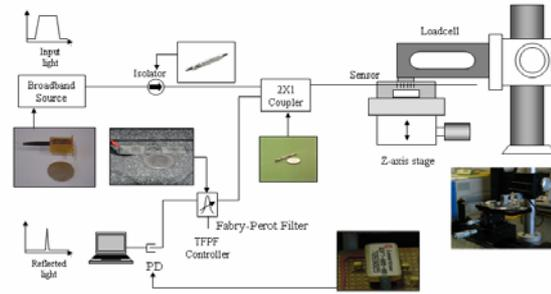
**Figure 10** Calibration system of prototype sensor
