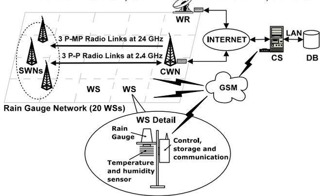
**Figure 1:** Weather station data Acquisition System (WAS) structure for the rain gauge network.
