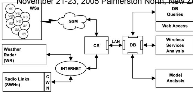
Figure 5: WAS architecture and database interfaces.
