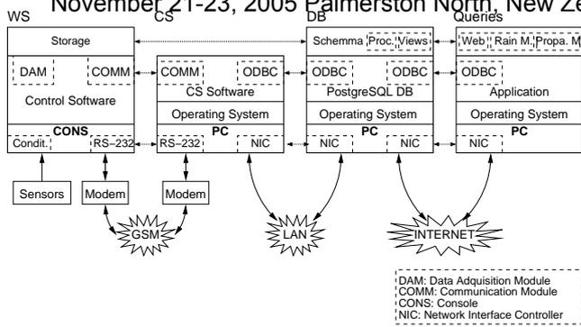
**Figure 7:** Communication example between elements, interfaces and layers.
