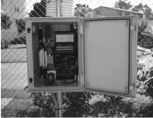
**Figure 3:** WS data acquisition and communications system assembled in the protection box.
