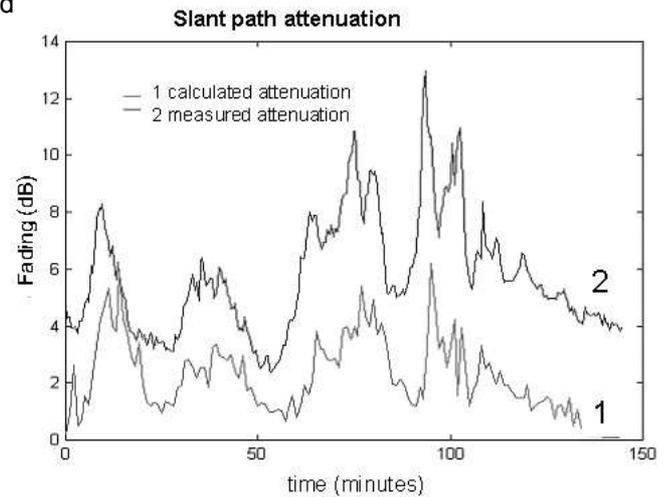
**Figure 8:** Comparison between measured and computed attenuation for the same radio link. Barcelona ITALSAT.  $41^\circ$  elevation, 39.6 GHz.
