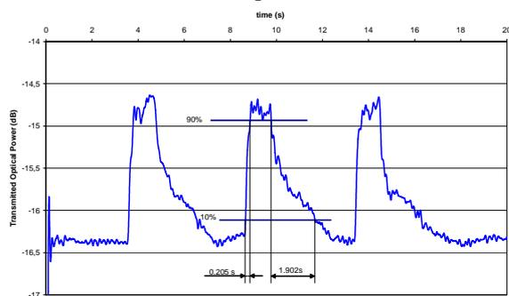
Figure 7. Response of the TOF sensor to human breathing.
