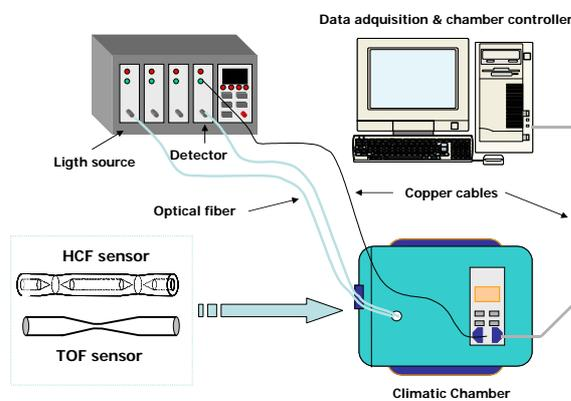
Figure 3. Experimental set-up to characterize the humidity sensors proposed
