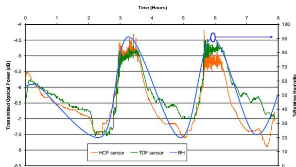
Figure 6. Humidity response comparison between a HCF and a TOF humidity based sensor at a wavelength of 1310 nm.
