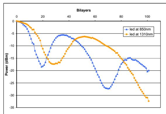
Figure 5. HCF based sensor transmitted optical power as a function of the thickness coating at two different wavelengths 1310 nm and 1550 nm.
