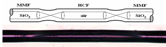
Figure 2. Profile and photograph of a HCF based structure
