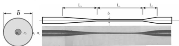
Figure 1. Profile and photograph of a TOF based structure.
