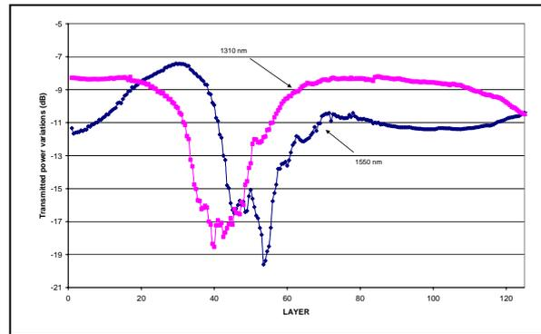
Figure 4. TOF based sensor transmitted optical power as a function of the thickness coating at two different wavelengths 1310 nm and 1550 nm
