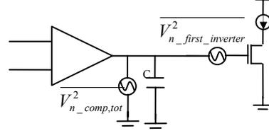
**Figure 7:** Noise model including the first inverter stage
