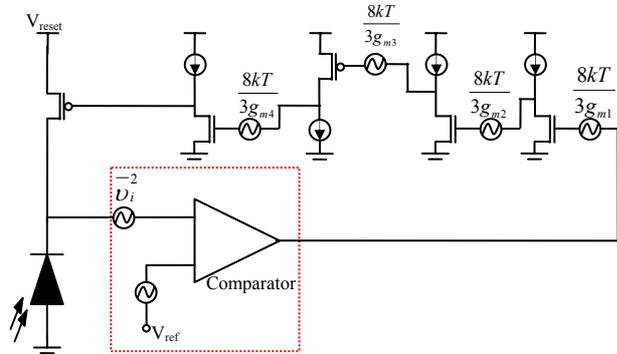
**Figure 6:** Noise model for the HDR pixel
