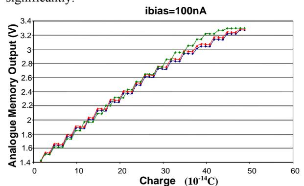
**Figure 4:** Analogue memory simulations (Red: 10  $\mu$ s pulse at beginning of exposure, Blue: 10  $\mu$ s pulse at end of exposure, Green: uniform illumination)
