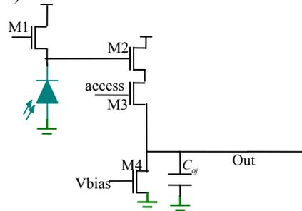
**Figure 8:** 3T voltage-mode pixel schematic
