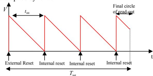
**Figure 1:** High dynamic sensor: pixel operation voltage output
