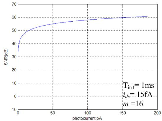
Figure 10: Signal-to-Noise Ratio vs. photocurrent
