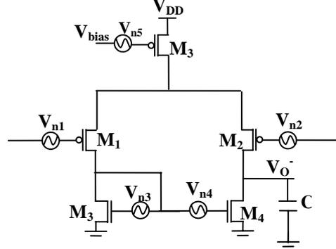
**Figure 5:** Differential pair noise model
