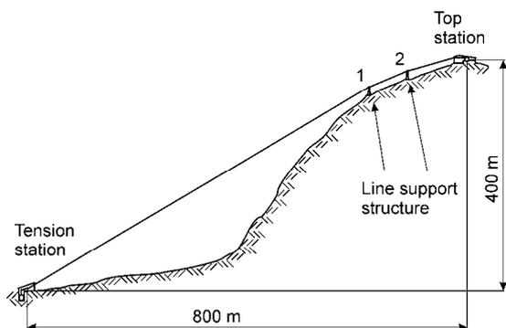
**Figure 4:** Longitudinal section of Lünersee ropeway.
