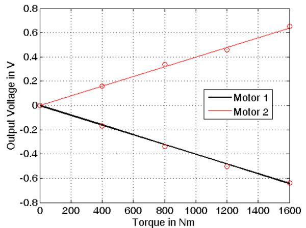
Figure 9: Calibration results of measurement chain.
