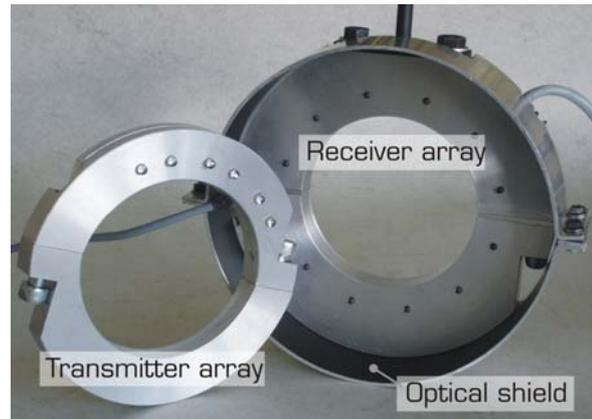
**Figure 2:** Housing of the IR array units.
