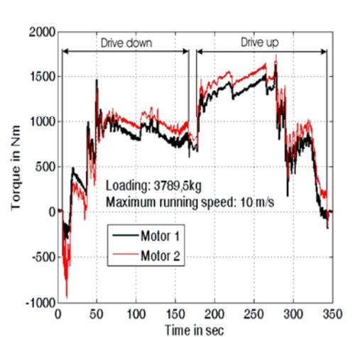
Figure 10: Example of the measuring results obtained with the described system.
