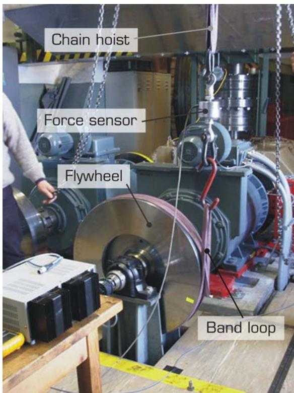
Figure 8: Arrangement for the calibration of the measurement chain.
