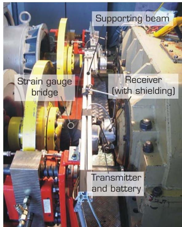
**Figure 6:** Measurement application on both shafts.
