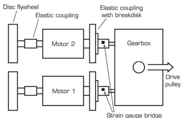
**Figure 5:** Block diagram of the drive system.
