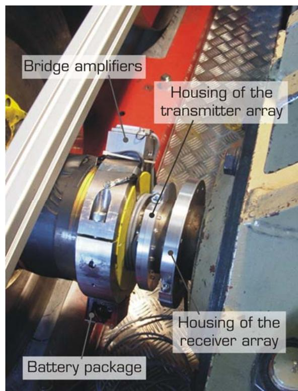
**Figure 7:** Details of the application on one driving shaft (without optical shield).
