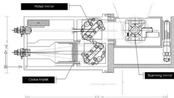
Figure 1: Scheme of ITR optical head.
