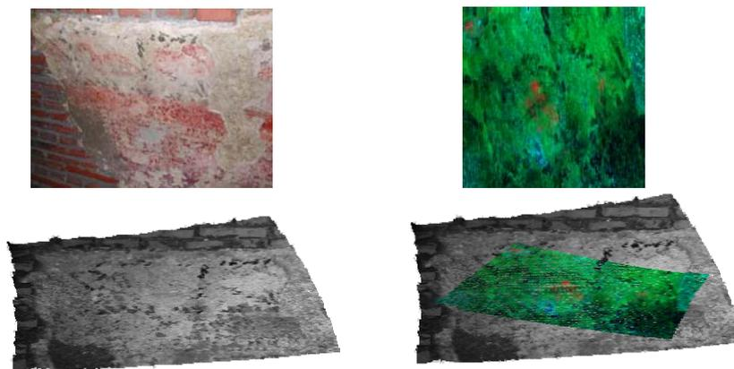
**Figure 4:** An example of multi-sensor data integration. Top left: photograph of the target – a wall in a Byzantine crypt in Constanta (Romania). Top right: LIF data, providing combined information about the fluorescence intensity on three channels at 580 nm (R), 532 nm (G) and 450 nm (B). Bottom left: 3D model. Bottom right: LIF data superimposed onto the 3D model.
