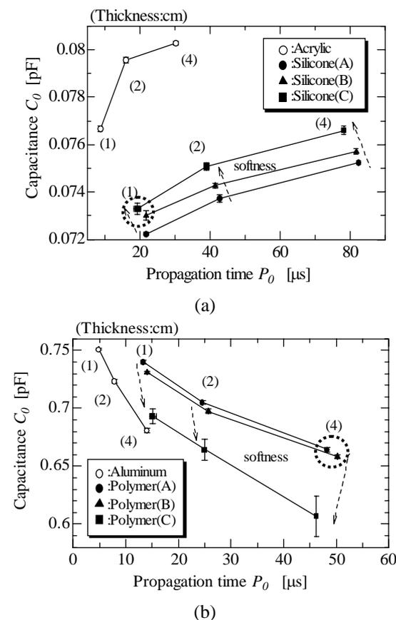
Figure 3: Experimental results. (a)Relationship between capacitance and propagation time in the case of silicone rubber and acrylic resin. (b)Relationship between capacitance and propagation time in the case of aluminium and acrylic resin.
