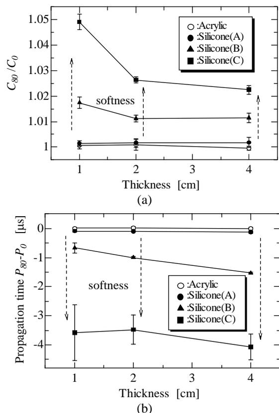
**Figure 4:** Changed values of capacitance and propagation time between two kinds of contact conditions in case of materials of acrylic resin and silicone rubber. (a) Measurement result of capacitance. (b) Measurement result of propagation time.
