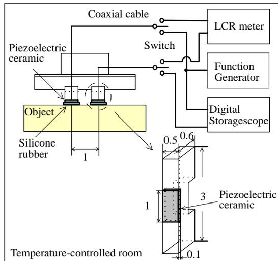
Figure 2: Schematic diagram of measurement system using proposed touch sensor.
