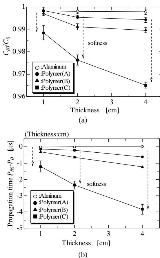
**Figure 5:** Changed values of capacitance and propagation time between two kinds of contact conditions in case of materials of aluminium and polymer gel. (a) Measurement result of capacitance. (b) Measurement result of propagation time.
