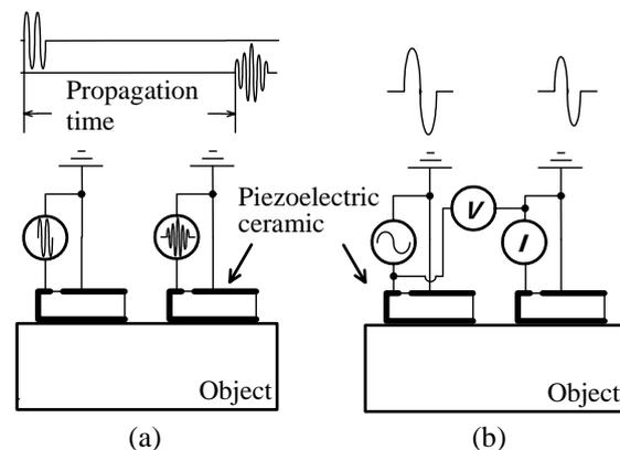
**Figure 1:** Measurement method of proposed touch sensor. (a) Measurement of ultrasonic property. (b) Measurement of electrical property.
