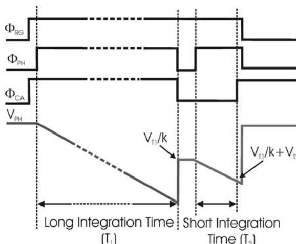
Figure 10: Timing diagram for dynamic range boosting.
