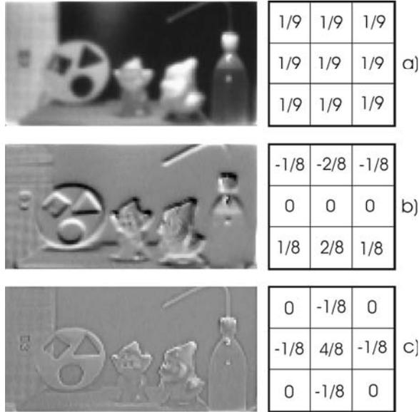
**Figure 5:** Examples of spatial filtering with time-based coefficient assignment: a) average filter; b) Sobel filter; c) Laplacian filter.
