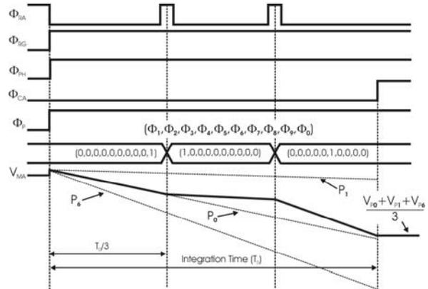
**Figure 3:** Timing diagram for an average filter over 3 pixels.
