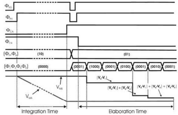
**Figure 6:** Timing diagram of switched-based approach referred to three pixel.
