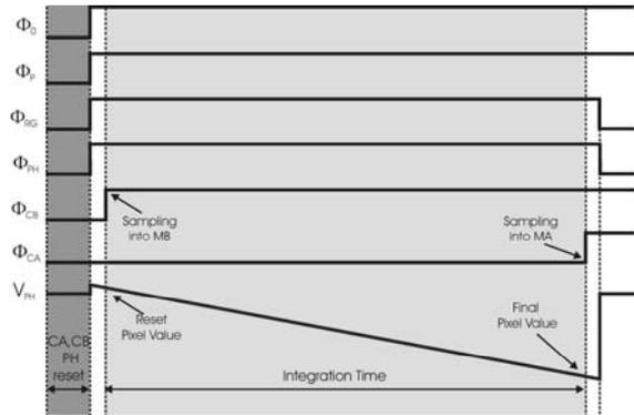
**Figure 2:** Timing diagram for camera mode operation.
