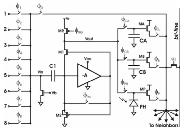
**Figure1:** Schematic of the pixel.
