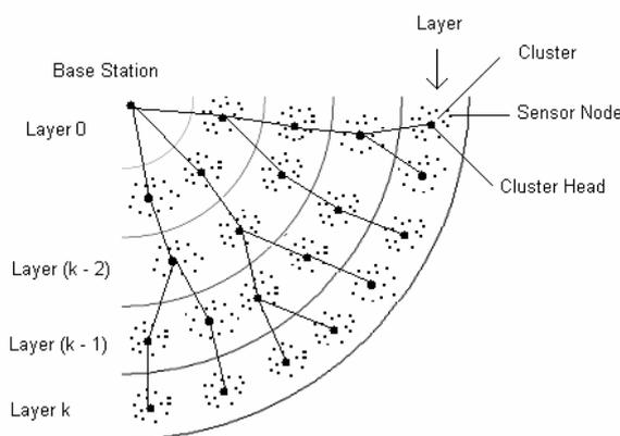
Figure 1. Hierarchical distribution of sensor nodes in Distributed Sensor Networks
