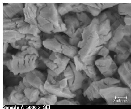
**Figure 2:** SEM of CeO<sub>2</sub> film at 5000 magnification
