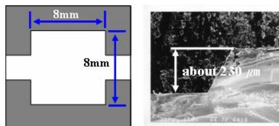
**Figure 5:** Mask layout of gas cell and SEM image of gas cell's cross section
