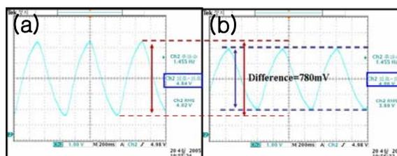
Figure 11: Response characteristic at 10,000ppm CO<sub>2</sub>
