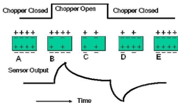
**Figure 2:** Pyroelectric effect representation in using chopper
