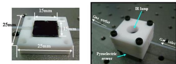
Figure 6: Fabricated gas cell and head part of sensor
