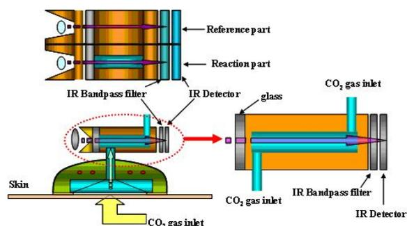
**Figure 4:** Schematic diagram of optical reaction chamber
