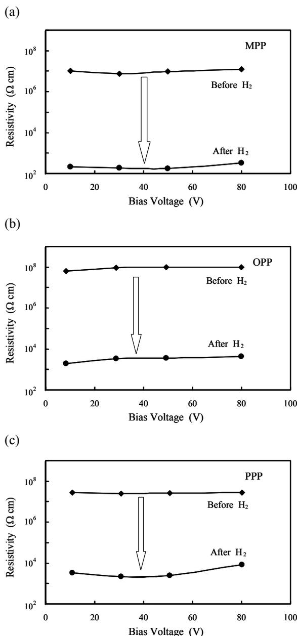
Figure 3: Changes in resistivity of the sensors before and after H<sub>2</sub> (100 %) as a function of applied voltage. (a) MPP, (b) OPP and (c) PPP.
