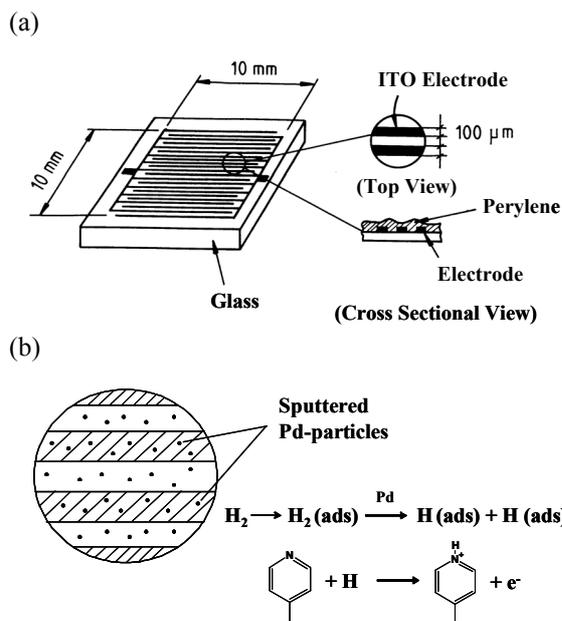
Figure 2: (a) Interdigital electrodes and (b) magnified Pd-sputtered electrodes.
