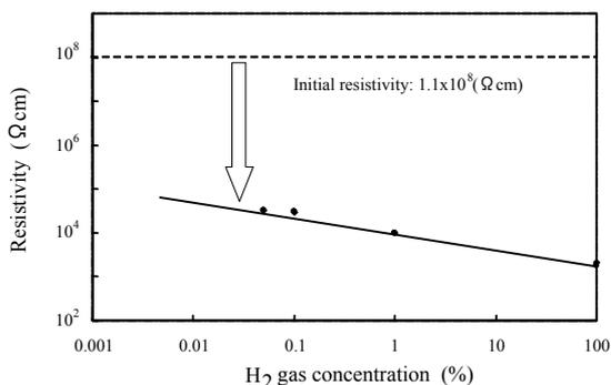
**Figure 4:** Log-log plot of the resistivity of the MPP sensor and H<sub>2</sub> concentration: 0.05, 0.1, 1 and 100 % H<sub>2</sub>.
