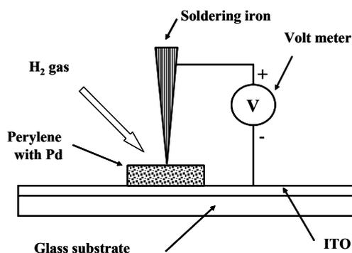
**Figure 6:** Experimental setup for measurements of Seebeck coefficient.
