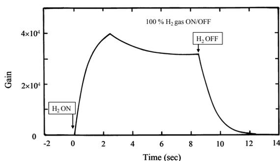
**Figure 5:** Build up and build down of the MPP sensor signal as a function of time.
