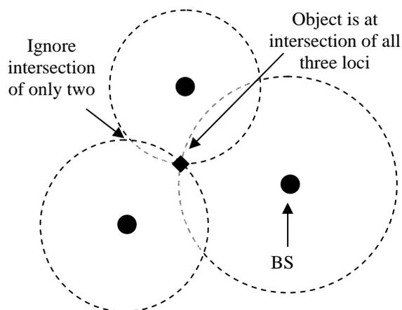
Figure 2: ToF positioning method.
