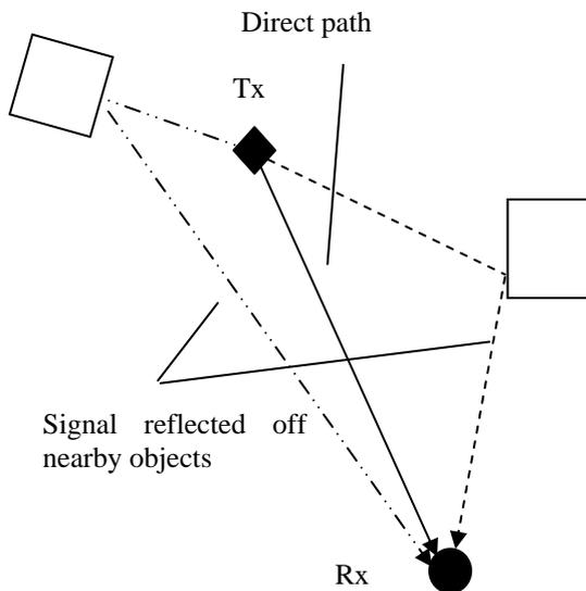
**Figure 3:** Base station experiencing multi-path fading.
