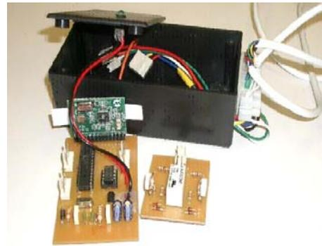
Figure 4: Tracking System Receiver Node
