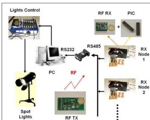
Figure 1: Diagram of test tracking network
