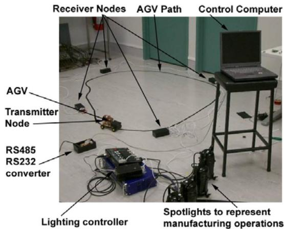
Figure 5: Tracking System Setup
