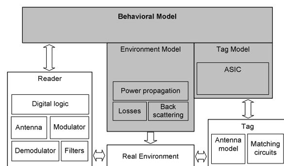
**Figure 2:** HIL verification of tag ASIC digital module design
