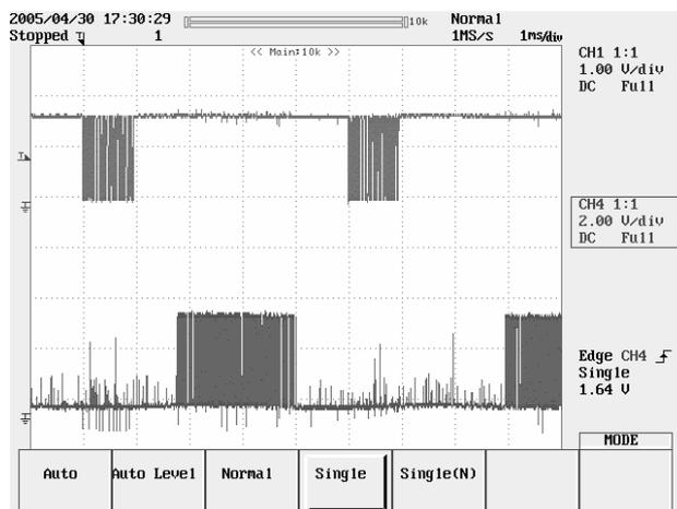
**Figure 9:** Commands send by the reader (upper signal) and the response from the tag emulator (lower signal)
