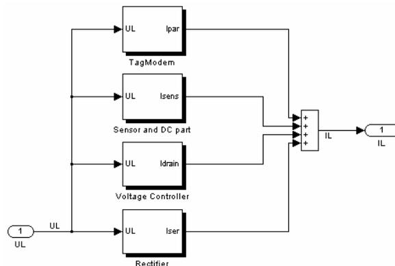
**Figure 5:** Block model of tag ASIC with a sensor module
