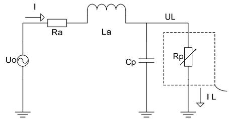
**Figure 4:** RLC circuit model of an RF-transponder
