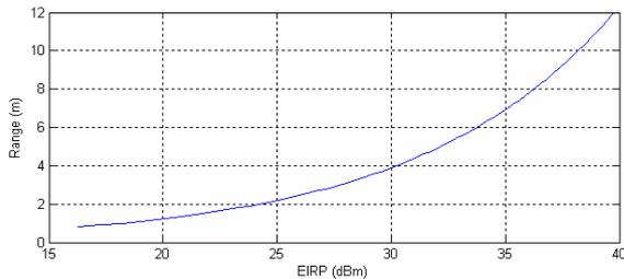
**Figure 3:** Achieved communication distance based on RF power transmitted by a reader
