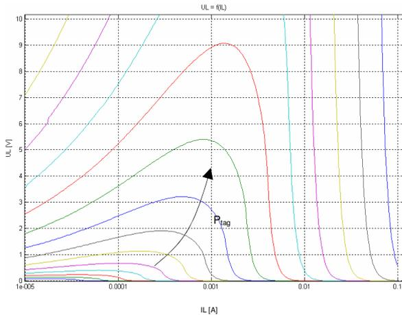
**Figure 7:** ASIC load voltage magnitude  $U_L$  as a function of load current magnitude  $I_L$  and RF input power magnitude  $P_{tag}$
