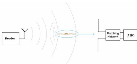
**Figure 1:** Principle of passive UHF transponders
