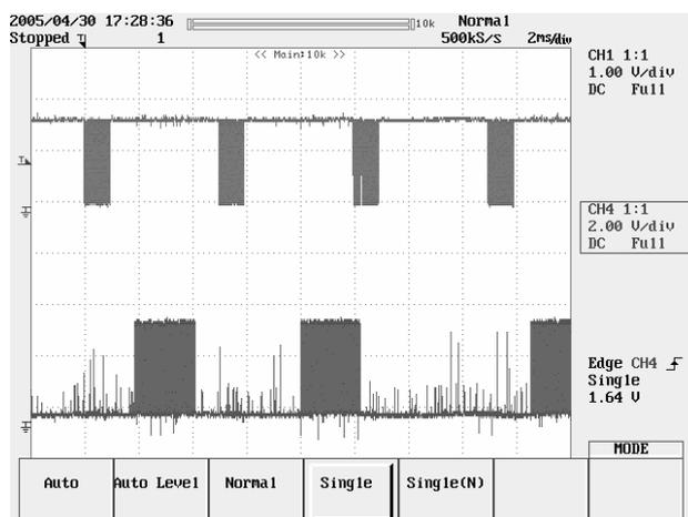
**Figure 10:** One reader command was missed due to the overlap of reader and tag data
