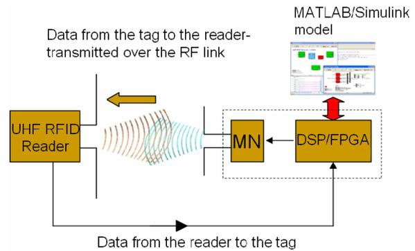
**Figure 8:** Concept of a HIL simulation architecture of an UHF RFID passive tag
