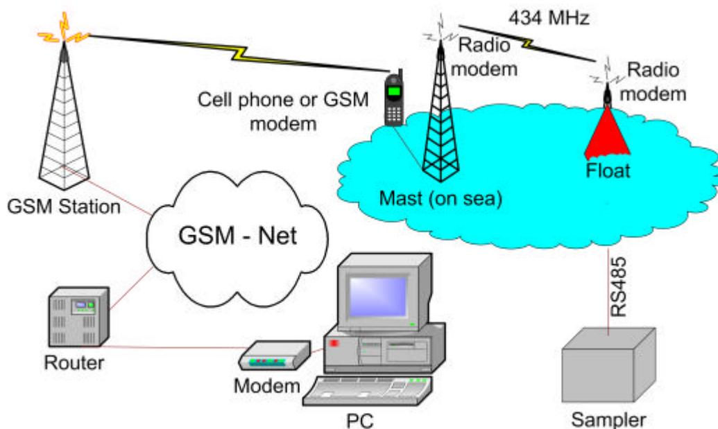
Figure 2: Schematic view of the remote controlled system
