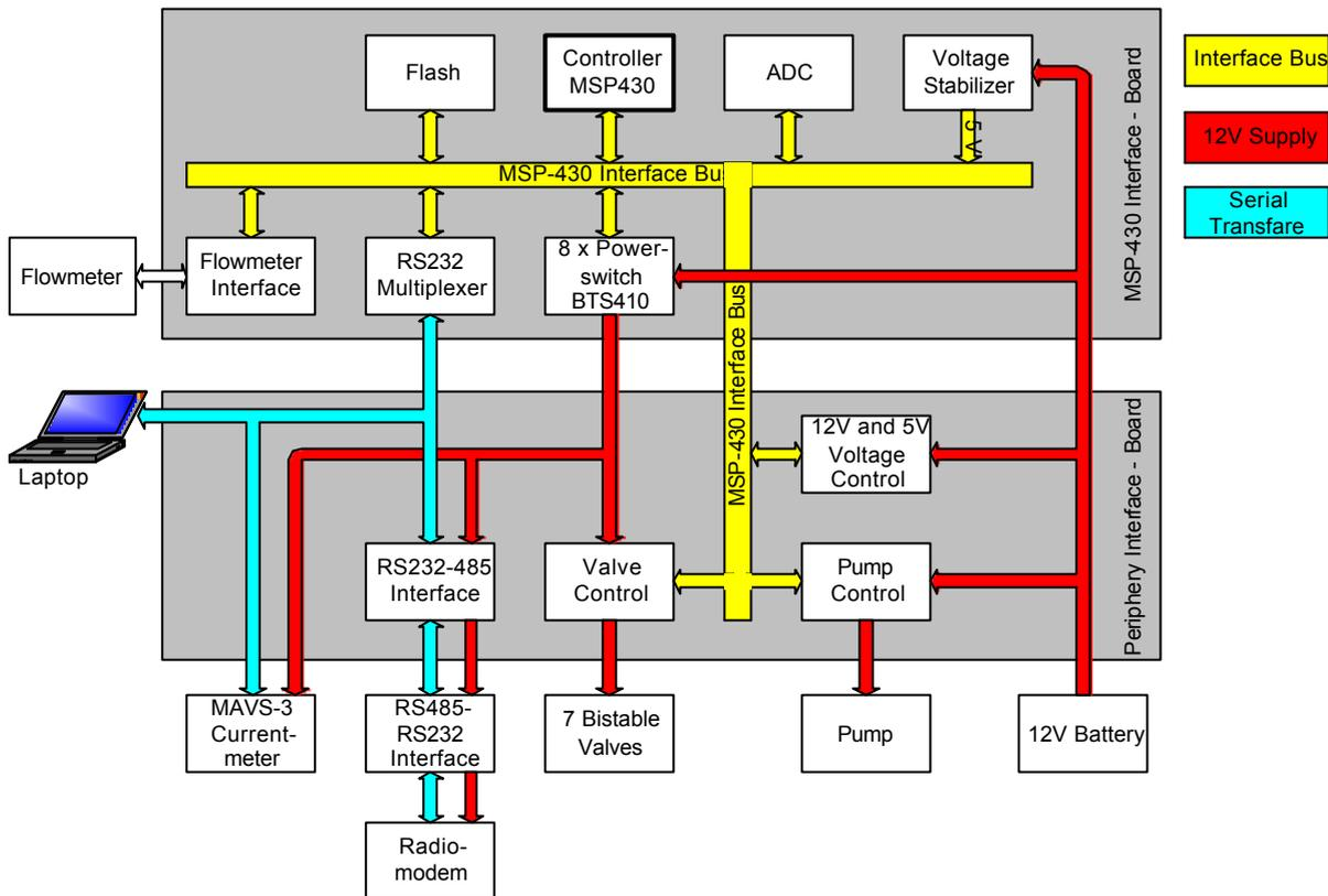
Figure 1: Block diagram of the filtration sampler
