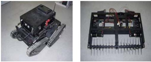
**Figure 1:** Mobile Robot vs. Demining Unit
