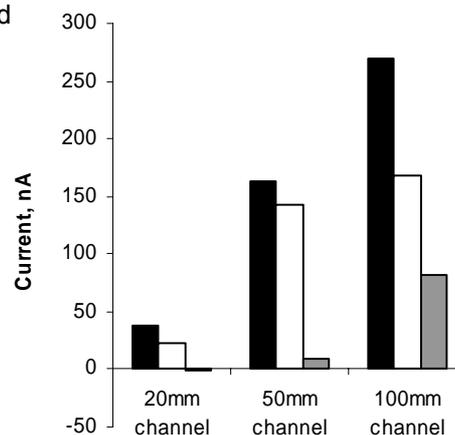
**Figure 5:** The detection of glucose (10 mM) in the acceptor stream of a microfluidic device. Currents generated in streams of various lengths, indicated on the X-axis, and at various flow rates:  $\blacksquare$  20  $\mu\text{l}/\text{min}$ ;  $\square$  40  $\mu\text{l}/\text{min}$ ;  $\blacksquare$  100  $\mu\text{l}/\text{min}$ .  $E_a = 600 \text{ mV vs. Ag/AgCl}$ .
