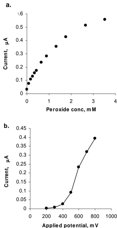
**Figure 3:** Currents generated **a.** by various concentrations of hydrogen peroxide in 0.1 M KCl;  $E_a = 600$  mV vs. Ag/AgCl, and **b.** by 1 mM hydrogen peroxide at various applied potentials. Channel length = 20 mm. Flow rate (a & b) =  $50\mu\text{l. min}^{-1}$ .
