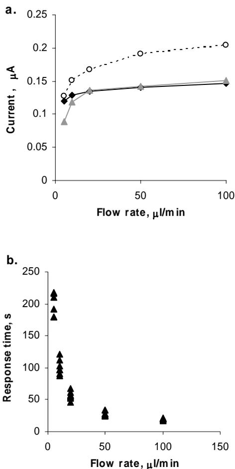
**Figure 4** a. Currents generated by 1 mM hydrogen peroxide in 0.1 M KCl at various flow rates. The curves are from replicates of devices, channel length = 20 mm. b. Relationship between flow rate and response time for the devices in a.
