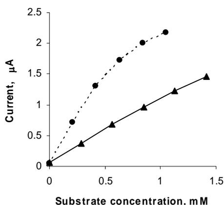
**Figure 2:** Currents generated at working electrodes by a flow ( $50\mu\text{l. min}^{-1}$ ) of various concentrations of catechol ( $\bullet$ ) or ferrocyanide ( $\blacktriangle$ ) in 0.1 M KCl.  $E_a = 600$  mV vs. Ag/AgCl. Channel length = 20 mm. Individual curves generated within the same device.
