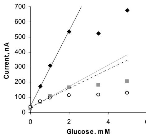
**Figure 6:** The relationship between current and glucose concentration in buffer and UF milk in an H-filter. Channel length = 100 mm. Flow rate = 20  $\mu\text{l}/\text{min}$ .  $\blacklozenge$  detection reagents and glucose mixed before being placed in device;  $\blacksquare$  glucose in buffer in donor stream;  $\circ$  glucose in spiked UF milk in donor stream (dashed line).
