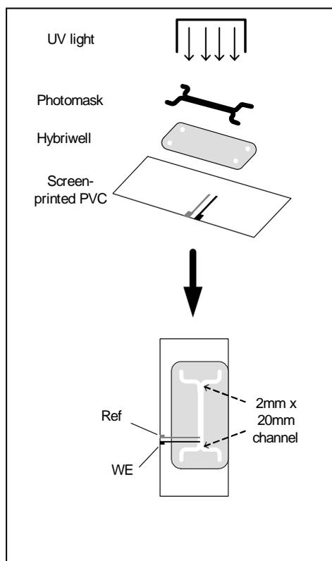
**Figure 1:** Schematic diagram illustrating the arrangement of parts during fabrication, and in the finished device.
