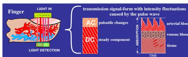
**Figure 1:** Principle- in vivo measurement on finger
