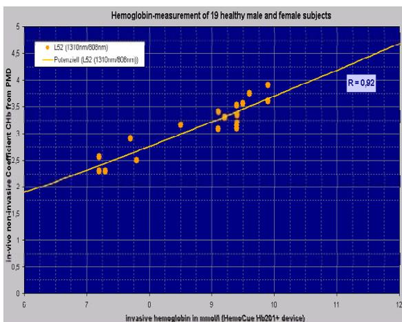
**Figure 5:** non-invasive Coefficient from PMD vs. invasive Haemoglobin measurements
