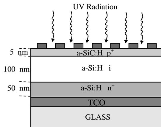
**Figure 1.** Structure of the device.
