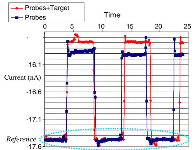
**Figure 5.** Sensor photocurrent as a function of time for single strand and hybridized DNA. Single-strand oligonucleotides has been functionalized on a glass substrate.
