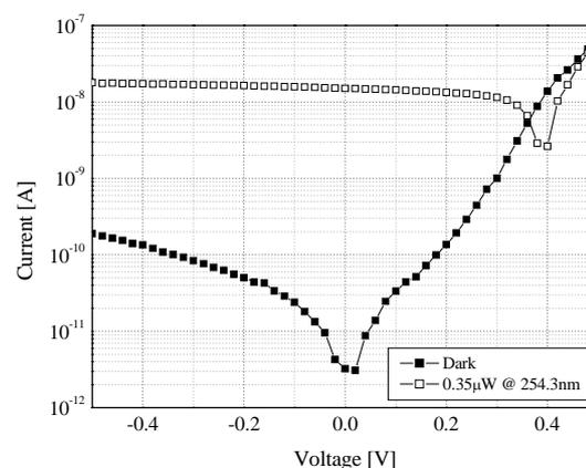
**Figure 3.** Current-voltage characteristics for the presented device in dark condition and under monochromatic light.
