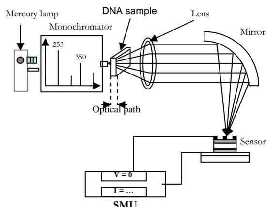
**Figure 2.** Experimental measurement set-up.
