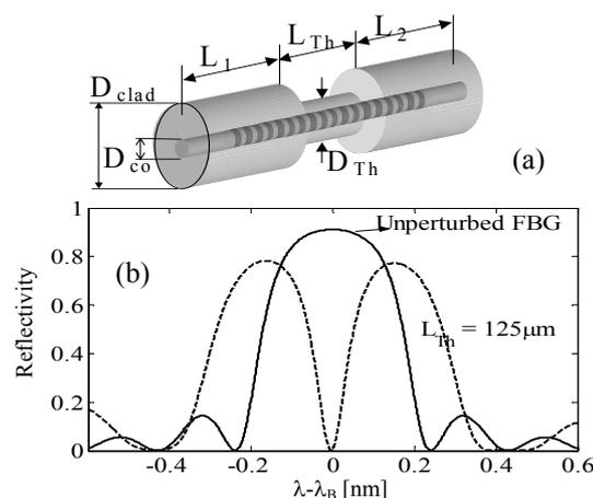
**Figure 8:** (a) Schematic diagram of the structure (not in scale), (b) spectral response in the case of full etching,  $L_{Th}=125\mu\text{m}$  and air as surrounding medium.
