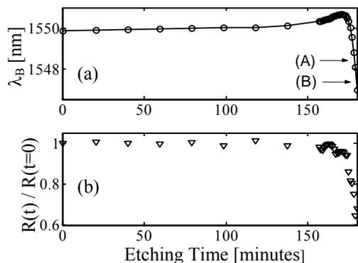
**Figure 3:** (a) Bragg wavelength and (b) maximum reflectivity percentage variation versus etching time.
