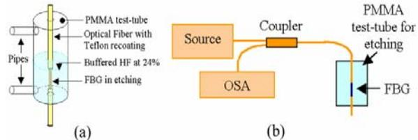
**Figure 2:** (a) Schematic of the PMMA package; (b) experimental set-up for refractive index measurements.
