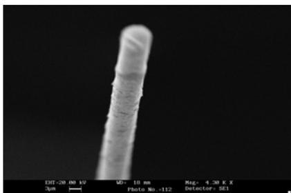
**Figure 4:** SEM photogram of the thinned optical fiber for the cladding diameter measurement.
