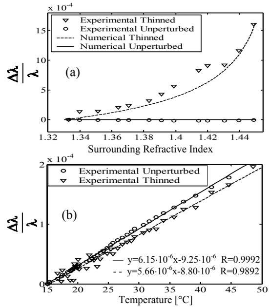
**Figure 7:** Relative shift for the thinned and the unperturbed wavelengths: (a) versus the external refractive index and (b) versus the temperature.
