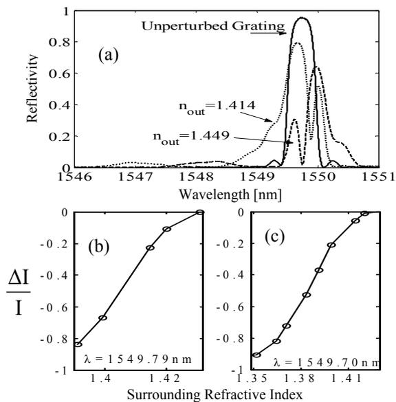
**Figure 9:** Experimental responses of the micro-structured grating versus the surrounding refractive index in case of  $L_{etch}=700\mu\text{m}$  and  $D_{etch}=10.5\mu\text{m}$ : (a) Reflected spectrum; (b) Reflectivity at  $\lambda=1549.79\text{nm}$ ; and (c) Reflectivity at  $\lambda=1549.70\text{nm}$ .
