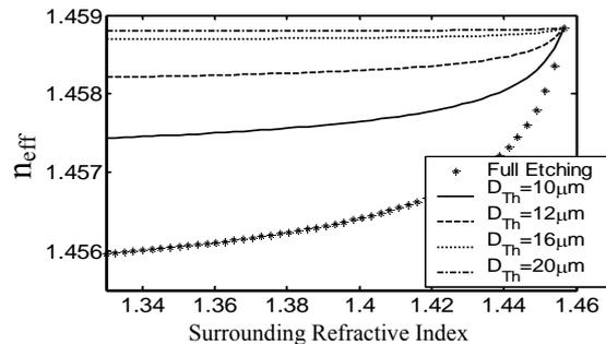
**Figure 1:**  $n_{eff}$  versus SRI for different cladding diameters.
