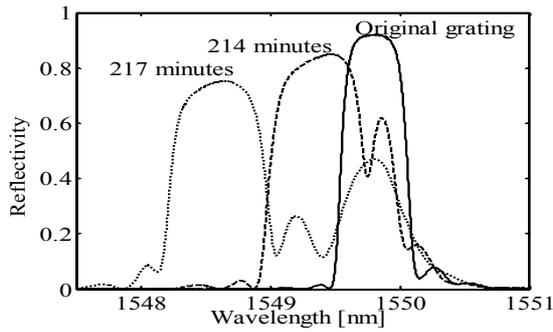
**Figure 6:** Reflected spectra during the etching process.
