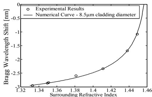
**Figure 5:** Wavelength shift of the reflected signal of the thinned Bragg filter (dotted line) and the numerical curve (solid line) with cladding diameter of  $8.5\mu\text{m}$  versus external medium.
