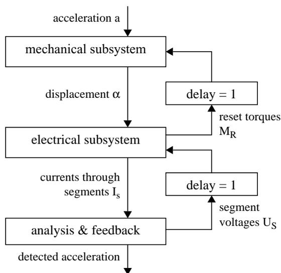
Figure 7: Structure of the sensor's SDF-model
