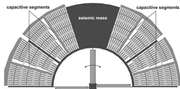
Figure 4: Sensor structure
