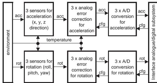
Figure 2: Analogue subsystem
