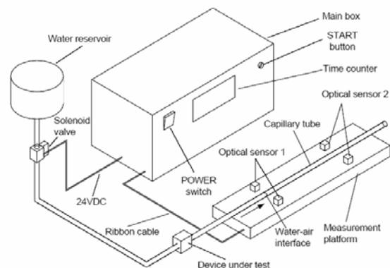
**Figure 3:** Perspective view of the OFMS. The two optical sensors detect the water-air interface to start/stop the time counter.
