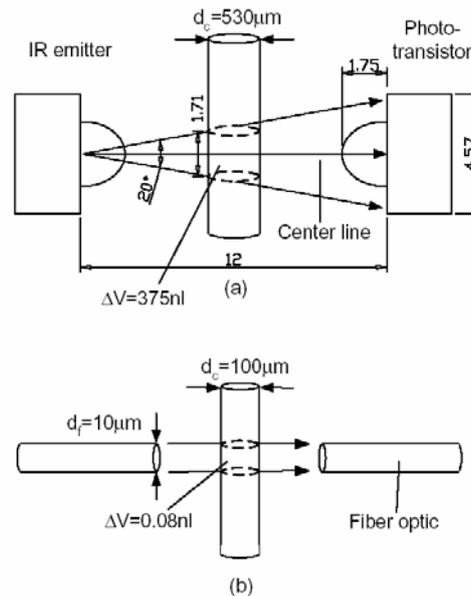
**Figure 8:** Volumetric resolution of the system. (a) Current configuration has volumetric resolution of 375 nl (b) Using finer capillary and replacing IR emitter-phototransistor by fiber optic improves the volumetric resolution to 0.08 nl.
