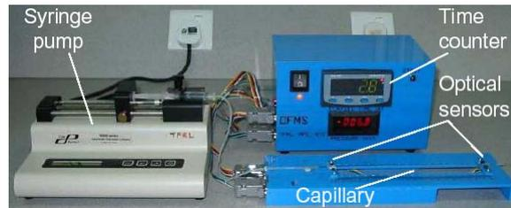
Figure 5: Calibration setup. The syringe pump drives a syringe to generate various precision flow rates, which are then compared to the measured data.
