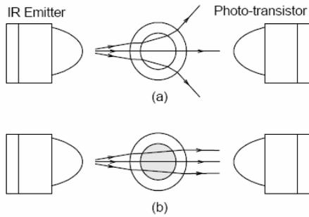
**Figure 1:** The principle of detecting liquid in a glass capillary using the difference of refractive indexes. (a) Air-filled capillary disperses light. (b) Liquid-filled capillary focuses light. (Adapted from [7])
