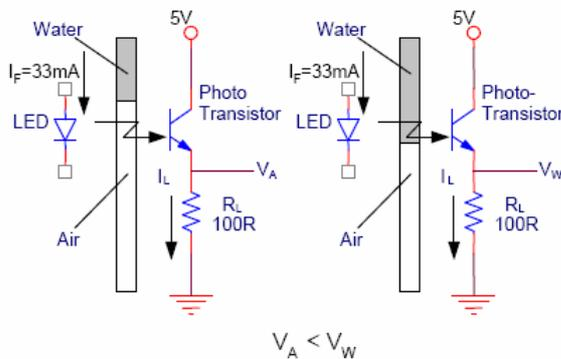
**Figure 2:** The phototransistor works in active mode, common-collector configuration. Water-filled capillary transmits infrared (880 nm) better than air-filled capillary. Therefore, the output voltage of water is higher  $V_w > V_a$ .
