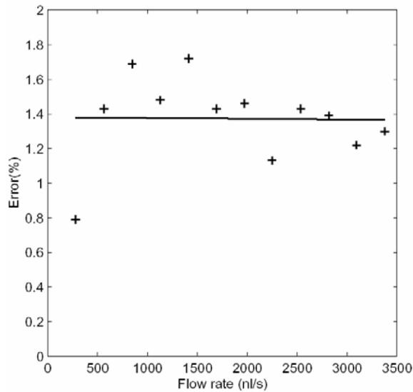
**Figure 7:** Errors (%) of the OMFS at different flow rates.
