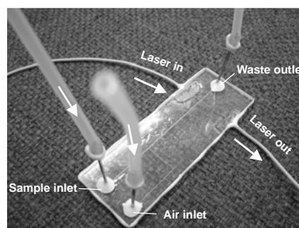
**Fig. 3:** The completed microfluidic sensor for dynamic surface tension measurement.
