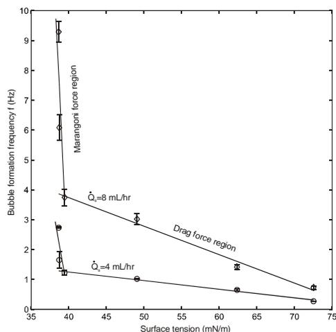
**Figure 7:** Measured bubble formation frequency as function surface tension.
