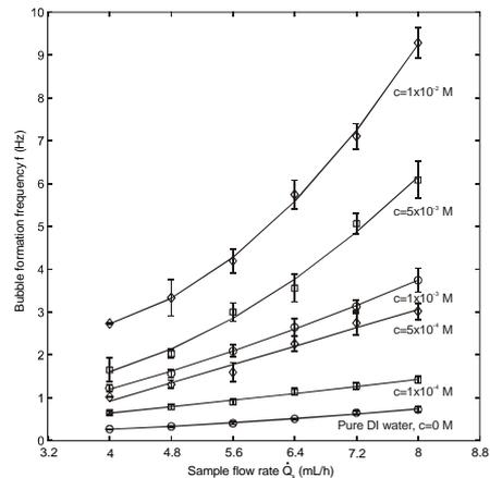
**Figure 5:** Measured bubble formation frequency as function of surface tensions at air flow rates of 1 mL/h and 2 mL/h.
