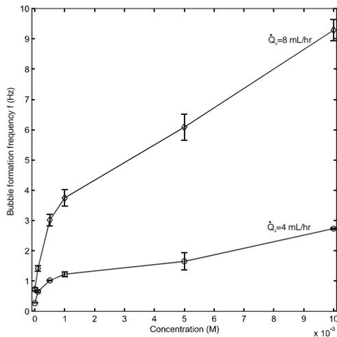
**Figure 6:** Measured bubble formation frequency as function surface tension.
