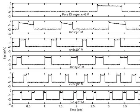
**Figure 4:** Typical bubble signals detected by the APD at an air flow rate of 1 ml/h (constant flow rate ratio  $\alpha=1:4$ )
