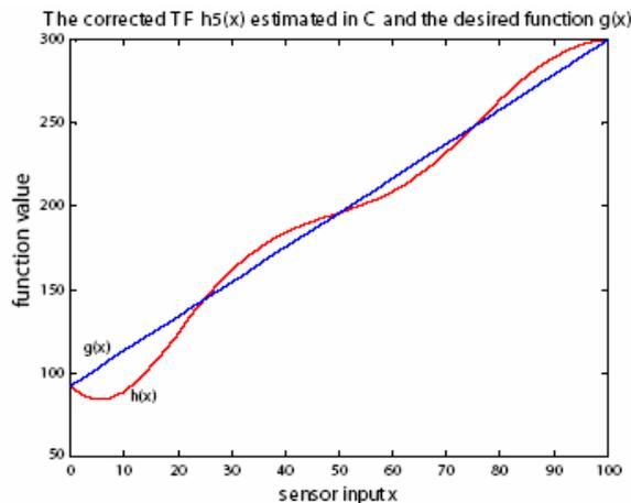
**Figure 9:** Corrected sensor TF  $h_5(x)$  of the sensor TF  $f_1$  using the PPC method with 5 points and the desired sensor TF  $g(x)$  plotted in MATLAB ( $x = \{0, 100, 50, 75, 25\}$ ).
