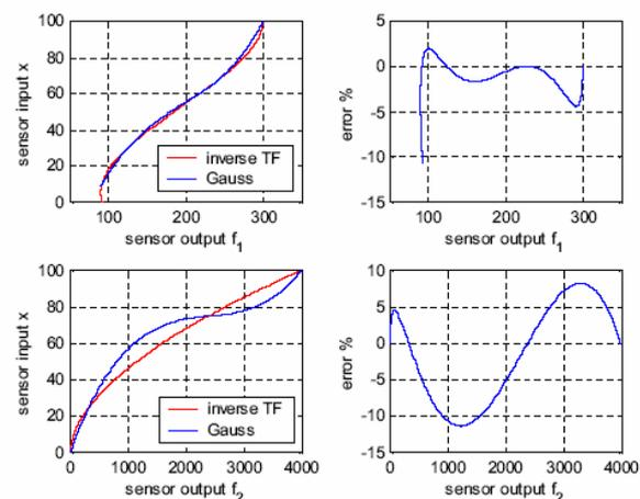
**Figure 7:** Interpolation with the third order polynomial using Gaussian elimination for calculating the coefficients and error percentage for the inverse transfer functions of the functions  $f_1$  and  $f_2$ .
