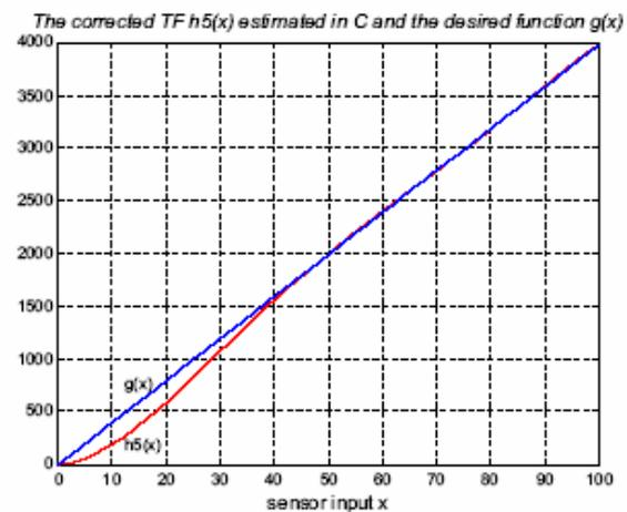
**Figure 12:** Corrected sensor TF  $h_5(x)$  of the sensor TF  $f_2$  using the PPC method with 5 points and the desired sensor TF  $g(x)$  plotted in MATLAB ( $x = \{0, 100, 68.04, 85.23, 46.294\}$  - equally spaced points on  $y$  axis).
