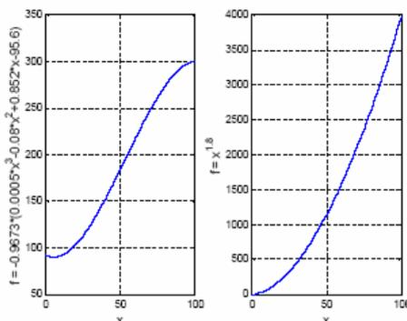
**Figure 5:** Sensor responses used as test functions described with  $f_1 = -0.9673(0.0005x^3 - 0.08x^2 + 0.852x - 95.6)$  and  $f_2 = x^{1.8}$ .
