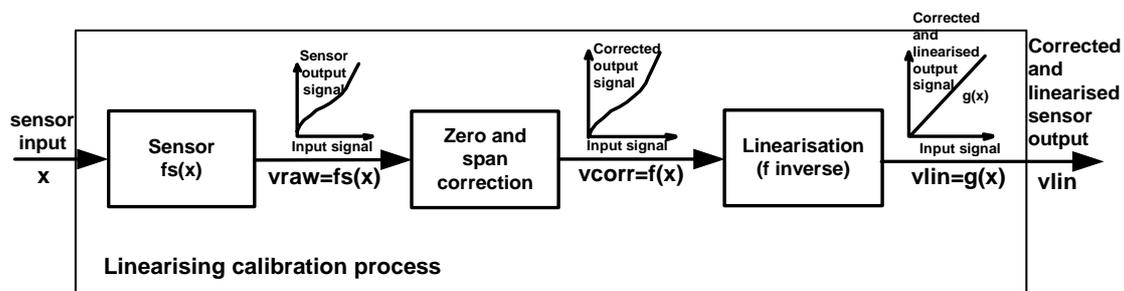
Figure 1: Linearising calibration process
