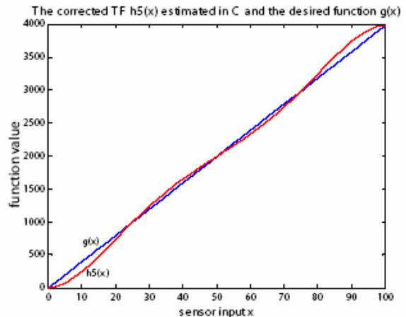
**Figure 11:** Corrected sensor TF  $h_5(x)$  of the sensor TF  $f_2$  using the PPC method with 5 points and the desired sensor TF  $g(x)$  plotted in MATLAB ( $x = \{0, 100, 50, 75, 25\}$  - equally spaced points on  $x$  axis).
