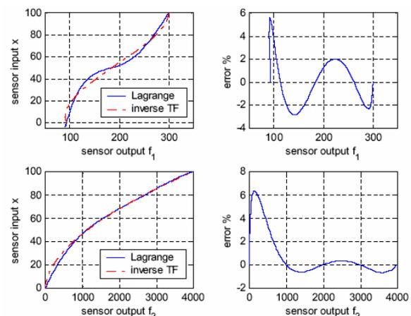
**Figure 8:** Lagrange polynomial interpolation and error percentage for the inverse transfer functions of the functions  $f_1$  and  $f_2$ .
