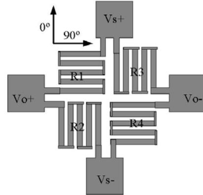
**Figure 3.** Schematic of a typical 0°-90° magnetoresistor used in this experiment. This sensor is a classic Wheatstone bridge.
