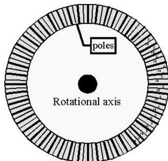
**Figure 6.** Schematic top view of a 48 pole pair ring magnet. This schematic shows how a ring magnet alternates the magnetic poles. Narrow lines represent north-south transitions.
