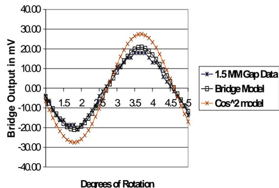
**Figure 8.** Comparison of experimental magnetoresistor bridge and the bridge model versus the angle of rotation for a ring magnet on a spindle. The model assumes that the field saturates the magnetoresistor and the external field rotates  $360^\circ$  every  $7.5^\circ$  of spindle rotation. The  $\cos^2 \theta$  model over-predicts the sensitivity of the 200 angstrom sensor.
