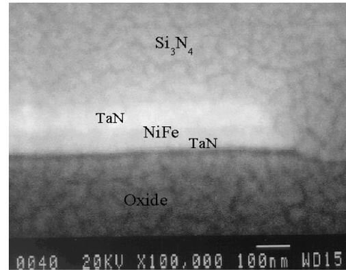
**Figure 4.** Cross-section of an AMR (anisotropic magnetoresistor) sensor element. Magnification 10000X.
