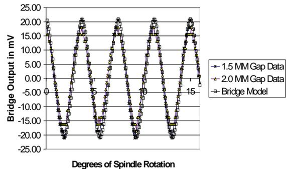
**Figure 7.** Comparison of experimental magnetoresistor bridge and the bridge model versus the angle of rotation for a ring magnet on a spindle. The model assumes that the field saturates the magnetoresistor and the external field rotates  $360^\circ$  every  $7.5^\circ$  of spindle rotation.
