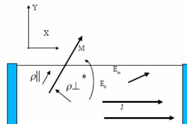
**Figure 1.** Schematic of an anisotropic magnetoresistor. The electric field due in this model is represented by an isotropic component and a magnetic component and the current density points in the x-direction.
