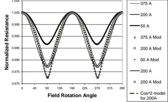
**Figure 2.** Magnetoresistance of three different saturated magnetoresistors versus the externally applied field direction. This graph shows the model fit for the 5nm, 20nm, 37.5nm and the 20nm  $\cos^2 \theta$  fit. It appears that the  $\cos^2 \theta$  model has the periodicity but not the shape of the data.
