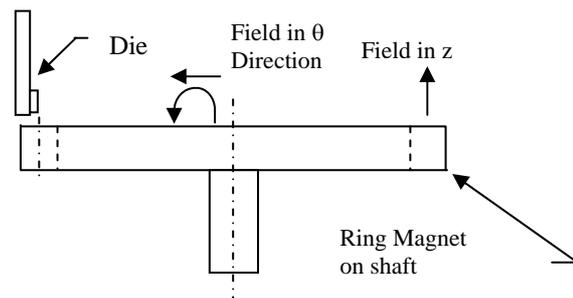
**Figure 5.** Ring Magnet test structure. The ring magnet consists of 48 pole pairs. The magnetic field in the area of the die (sensor bridge) rotates 360° for every North-South-North transition.
